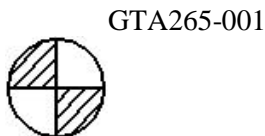
Figure 21.1 An example borehole where GTA265 represents the project number and 001 represents the sequential number.
